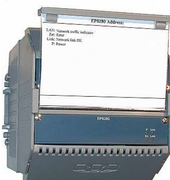
Figure 9. The inlay card in the upper position shows the signal descriptions for the PIFA-unit in the lower position.
