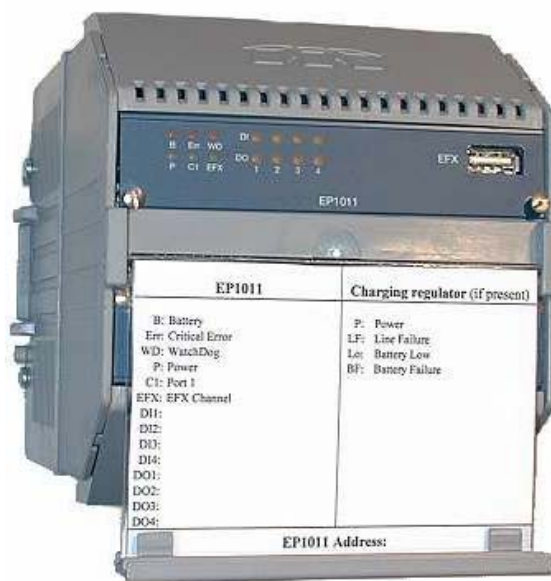
Figure 9. The inlay card in the upper position shows the signal descriptions for the PIFA-unit in the lower position.
